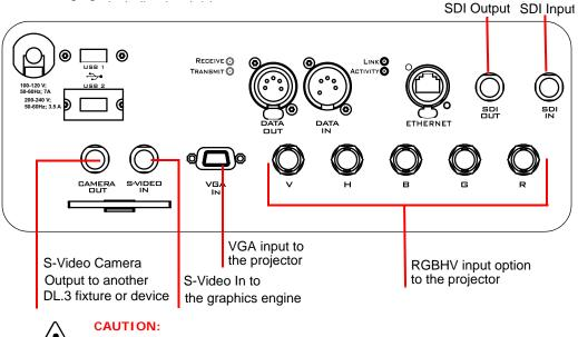
To avoid damaging the fixture and voiding the warranty, do not physically connect to the RGBHV and VGA inputs at the same time.
