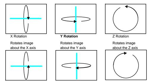
The Rotation parameters' suggested default values are the midpoint of the 16-bit DMX value range, which is equal to no rotation. Increasing the DMX value from the midpoint indexes the object in a clockwise direction. Reducing the DMX value below the midpoint indexes the object in a counterclockwise direction.
