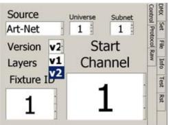
Art-Net—Data is transmitted over Ethernet cables using the Art-Net protocol. Set the number of DMX Universes (and DL.3 Ethernet Subnetworks containing this fixture from 0–16).
