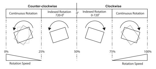
NOTE: Global and Graphic Effects Mode parameters contain a Prerotation Translation effect option. When a Global or Graphic Effects Mode DMX value = 102, you can use the Effect Modifier parameters to locate the image in a virtual three dimensional space. Applying the Rotation parameters then cause the image to orbit around the selected axis from that location, see Prerotation Translation on page 220.
