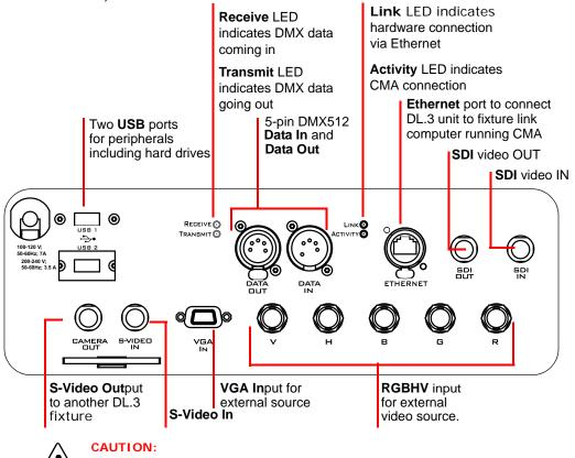
To avoid damaging the fixture and voiding the warranty, do not physically connect to the RGBHV and VGA inputs at the same time.
