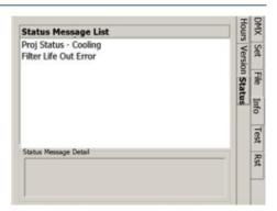
returns to the large format error display should there be any new messages to be displayed or if there is a persistent error. A persistent error is a case where the error condition continues to occur.
