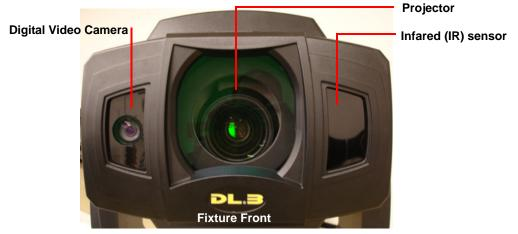
The camera is mounted on the front of the unit near the projector iris to point wherever the fixture is directed.
